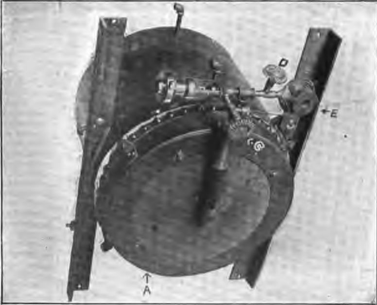
Fig. 221.—Base of Boiler and Burner of the "Reading" Carriage, showing regulator and starter coil in position. A is the burner case; C, the hand-wheel controlling the valve to the mixing tube; D, the hand-wheel controlling the valve to the auxiliary vaporizing coil; E; F, the diaphragm regulator.
